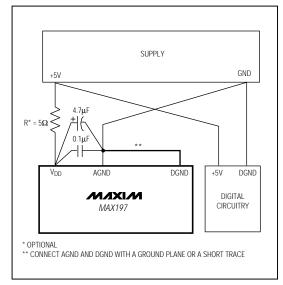
Figure 12. Power-Supply Grounding Connection
