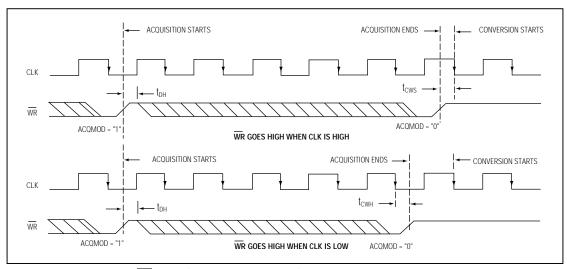
Figure 8b. External Clock and  $\overline{\textit{WR}}$  Timing (External Acquisition Mode)
