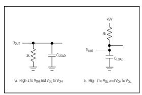
Figure 2. Load Circuits for Enable Time
