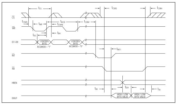
Figure 6. Conversion Timing Using External Acquisition Mode
