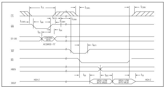
Figure 5. Conversion Timing Using Internal Acquisition Mode
