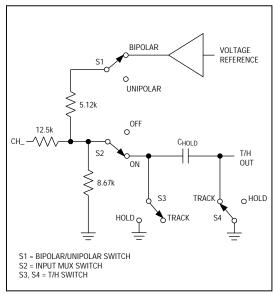
Figure 4. Equivalent Input Circuit
