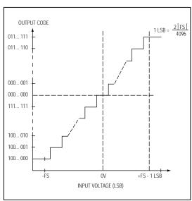
Figure 11. Bipolar Transfer Function
