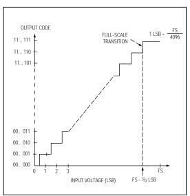
Figure 10. Unipolar Transfer Function
