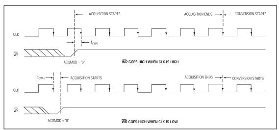
Figure 8a. External Clock and WR Timing (Internal Acquisition Mode)
