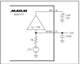
Figure 9c. External Reference, Reference at REFADJ
