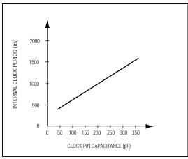
Figure 7. Internal Clock Period vs. Clock Pin Capacitance
