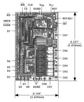
TRANSISTOR COUNT: 2956 SUBSTRATE CONNECTED TO GND
