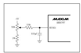
Figure 1. Reference-Adjust Circuit
