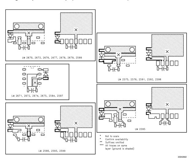
FIGURE 2. Recommended Layout Starting Points
