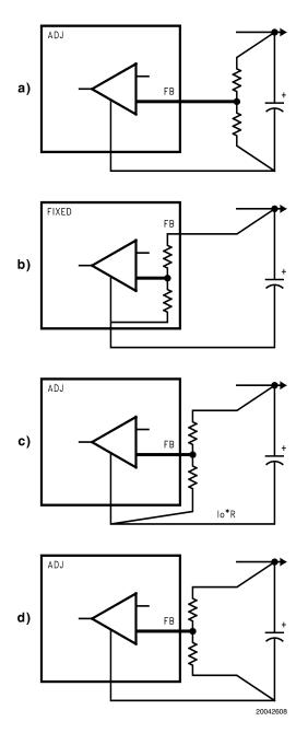
FIGURE 5. Feedback Traces (bold lines susceptible to noise)
