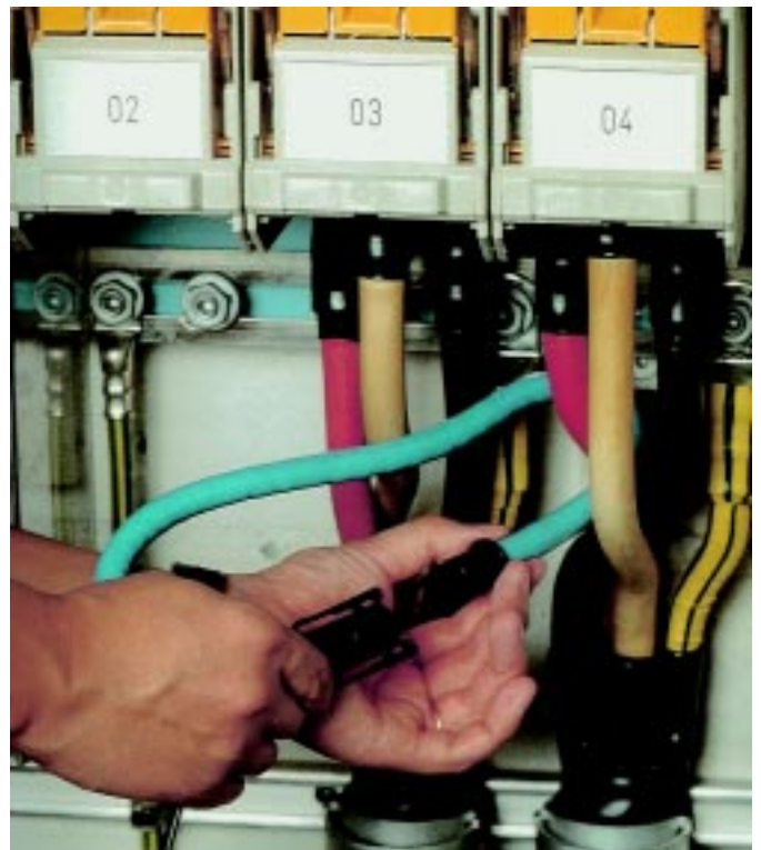
Fig. 18 The flexible current probe LEM-flex can measure AC currents and be wrapped around one or several conductors.
