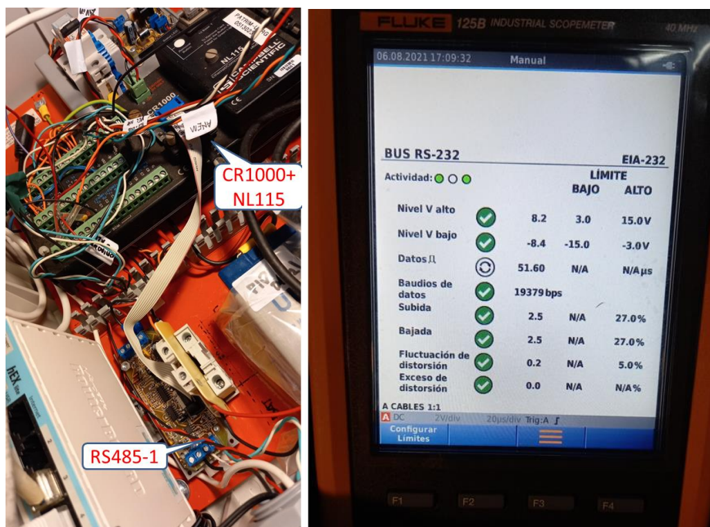
Figure 8 – CR1000 datalogger connected via its RS232 port to an RS485-1 converter board (left), configured as RS232-to-RS485 and linked the Arduino auxiliary system. The bus health test (right) was taken with a single probe connected to the TX0* output referenced to GND, using UNPA's F125B Scopemeter
